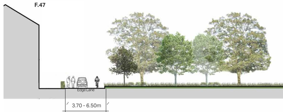
**Figure 47:** Diagram of a suitable edge lane used at the edge of the built-up areas to act as a transition into the countryside.
